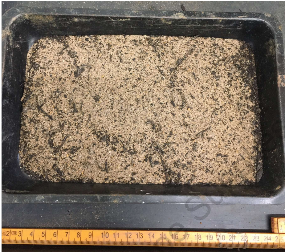
Plate 1: High Permeability Turfsoil (S) Sample
